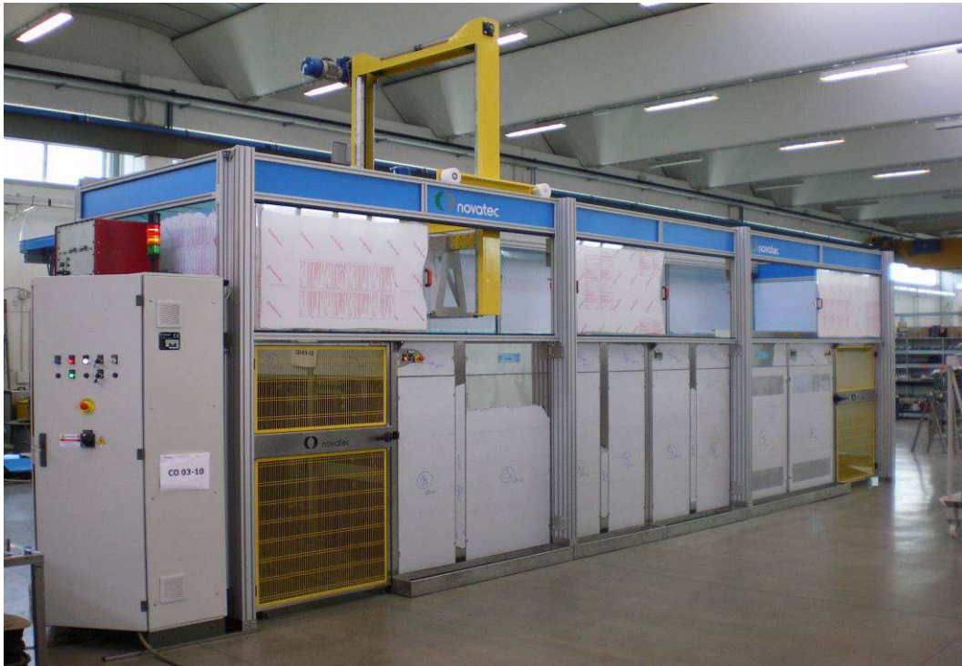
Automated ultrasonic cleaning system for moulds
