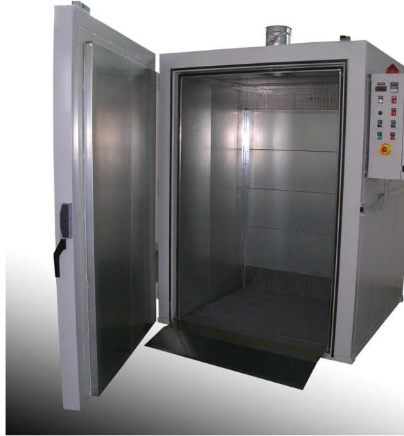
This oven has been specifically designed for the drying of varnish; it is provided with a heat exchanger, installed next to the drying room, which provides for the thermo exchange by means of an electro-ventilator.
