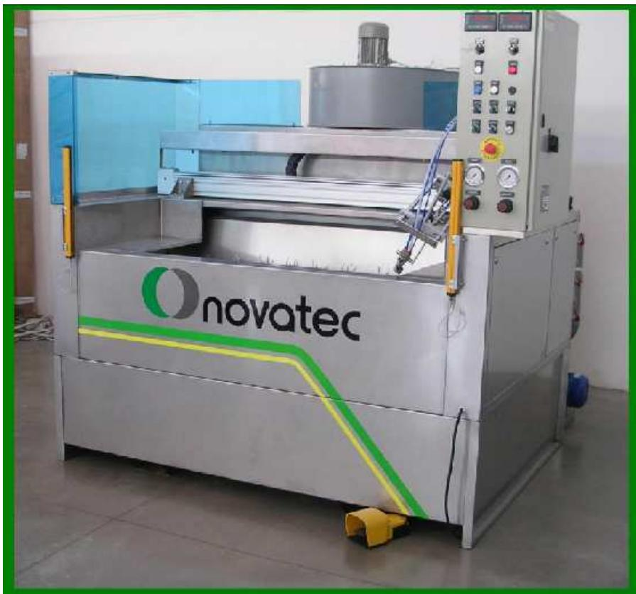
**BOOTH:** Entirely made of stainless steel AISI 304, it is equipped with double water veil, collecting tank, drops separator and air filter.
