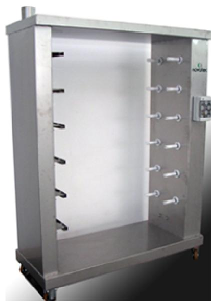
Varnish drying modules type GTR are used to keep just varnished frames in continuous rotation. This movement favours the homogeneous varnish laying before drying phase.
